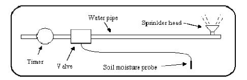
Figure 2: A closed-loop sprinkler system.
