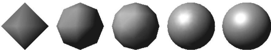
Figure 6.12 Representation of a sphere with different tessellations
