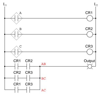
Either one of these circuits will adequately perform the task of operating the incinerator waste valve based on a flame verification from two out of the three flame sensors. At minimum, this is what we need to have a safe incinerator system. We can, however, extend the functionality of the system by adding to it logic circuitry designed to detect if any one of the sensors does not agree
