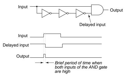
This circuit may be converted into a negative-edge pulse detector circuit with only a change of the final gate from AND to NOR:
