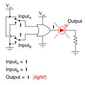
A condition of any input being raised to a "high" logic level makes the OR gate's output go "high," thus energizing the LED for three out of the four input combination states.
