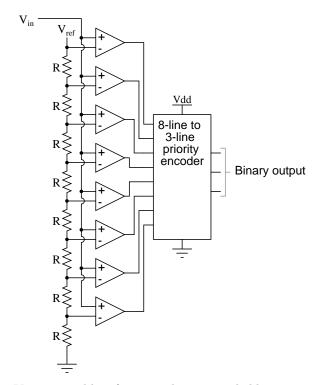
$V_{ref}$  is a stable reference voltage provided by a precision voltage regulator as part of the converter circuit, not shown in the schematic. As the analog input voltage exceeds the reference voltage at each comparator, the comparator outputs will sequentially saturate to a high state. The priority encoder generates a binary number based on the highest-order active input, ignoring all other active inputs.
