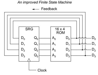
An analogy for the workings of such a device might be an array of post-office boxes, each one with an identifying number on the door (the address), and each one containing a piece of paper with the address of another P.O. box written on it (the data). A person, opening the first P.O. box, would find in it the address of the next P.O. box to open. By storing a particular pattern of addresses
