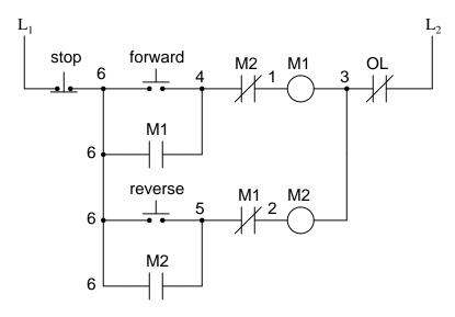
Now, if either forward or reverse circuits are latched, they may be "unlatched" by momentarily pressing the "Stop" pushbutton, which will open either forward or reverse circuit, de-energizing the energized contactor, and returning the seal-in contact to its normal (open) state. The "Stop" switch, having normally-closed contacts, will conduct power to either forward or reverse circuits when released.
