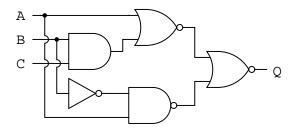
As always, our first step in simplifying this circuit must be to generate an equivalent Boolean expression. We can do this by placing a sub-expression label at the output of each gate, as the inputs become known. Here's the first step in this process:
