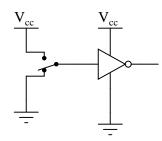
" $V_{cc}$ " stands for the constant voltage supplied to the collector of a bipolar junction transistor circuit, in reference to ground. Those points in a gate circuit marked by the label " $V_{cc}$ " are all connected to the same point, and that point is the positive terminal of a DC voltage source, usually 5 volts.
