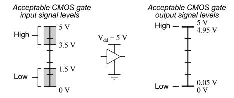
It should be obvious from these figures that CMOS gate circuits have far greater noise margins than TTL: 1.45 volts for CMOS low-level and high-level margins, versus a maximum of 0.7 volts for TTL. In other words, CMOS circuits can tolerate over twice the amount of superimposed "noise" voltage on their input lines before signal interpretation errors will result.
