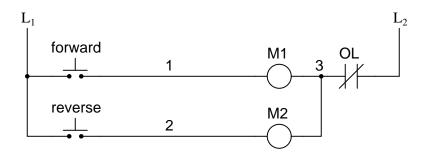
Take note of the normally-closed "OL" contact, which is the thermal overload contact activated by the "heater" elements wired in series with each phase of the AC motor. If the heaters get too hot, the contact will change from its normal (closed) state to being open, which will prevent either contactor from energizing.
