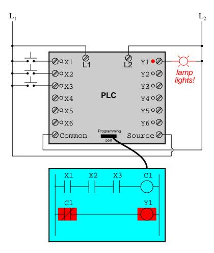
In this circuit, the lamp will remain lit so long as any of the pushbuttons remain unactuated (unpressed). To make the lamp turn off, we will have to actuate (press) *all* three switches, like this:
