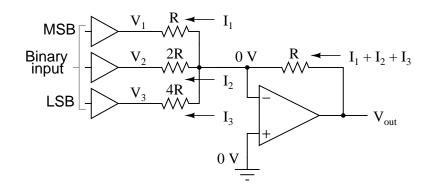
If we chart the output voltages for all eight combinations of binary bits (000 through 111) input to this circuit, we will get the following progression of voltages:
