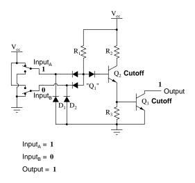
In any case where there is a grounded ("low") input, the output is guaranteed to be floating ("high"). Conversely, the only time the output will ever go "low" is if transistor  $Q_3$  turns on, which means transistor  $Q_2$  must be turned on (saturated), which means neither input can be diverting  $R_1$  current away from the base of  $Q_2$ . The only condition that will satisfy this requirement is when both inputs are "high" (1):
