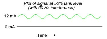
The above example is a bit exaggerated, but the concept should be clear: any electrical noise introduced into an analog measurement system will be interpreted as changes in the measured quantity. One way to combat this problem is to symbolize the tank's water level by means of a digital signal instead of an analog signal. We can do this really crudely by replacing the analog transmitter device with a set of water level switches mounted at different heights on the tank:
