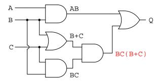
Finally, the output ("Q") is seen to be equal to the expression AB + BC(B + C):
