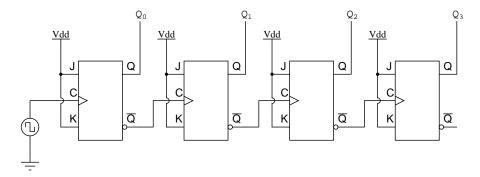
One way we could expand the capabilities of either of these two counter circuits is to regard the Q' outputs as another set of four binary bits. If we examine the pulse diagram for such a circuit, we see that the Q' outputs generate a *down*-counting sequence, while the Q outputs generate an *up*-counting sequence:
