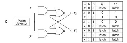
Only when the clock signal (C) is transitioning from low to high is the circuit responsive to the
