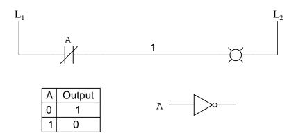
Now, the lamp energizes if the contact is *not* actuated, and de-energizes when the contact *is* actuated.
