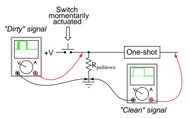
What if we only wanted a 10 second timed pulse output from a relay logic circuit, *regardless* of how many input pulses we received or how long-lived they may be? In that case, we'd have to couple a pulse-detector circuit to the retriggerable one-shot time delay circuit, like this:
