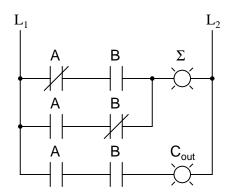
Either circuit is capable of adding two binary digits together. The mathematical "rules" of
