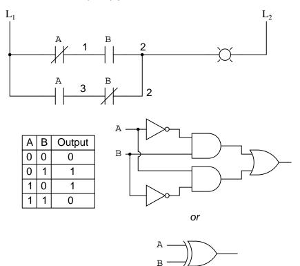
The top rung (NC contact A in series with NO contact B) is the equivalent of the top NOT/AND gate combination. The bottom rung (NO contact A in series with NC contact B) is the equivalent of the bottom NOT/AND gate combination. The parallel connection between the two rungs at wire number 2 forms the equivalent of the OR gate, in allowing either rung 1 *or* rung 2 to energize the lamp.
