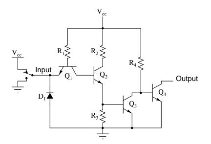
As before with the inverter circuit, the "high" input causes no conduction through the left steering diode of  $Q_1$  (emitter-to-base PN junction). All of  $R_1$ 's current goes through the base of transistor  $Q_2$ , saturating it:
