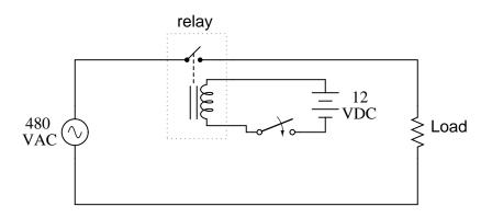
In the above schematic, the relay's coil is energized by the low-voltage (12 VDC) source, while the single-pole, single-throw (SPST) contact interrupts the high-voltage (480 VAC) circuit. It is quite likely that the current required to energize the relay coil will be hundreds of times less than the current rating of the contact. Typical relay coil currents are well below 1 amp, while typical contact ratings for industrial relays are at least 10 amps.
