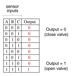
It does not require much insight to realize that this functionality could be generated with a three-input AND gate: the output of the circuit will be "high" if and only if input A AND input B AND input C are all "high:"
