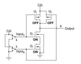
As with the TTL NAND gate, the CMOS NAND gate circuit may be used as the starting point for the creation of an AND gate. All that needs to be added is another stage of transistors to invert the output signal:
