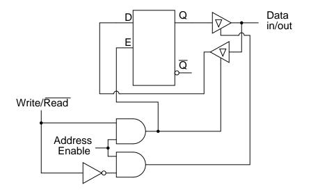
When the address enable input is 0, both tristate buffers will be placed in high-Z mode, and the latch will be disconnected from the data input/output (bus) line. Only when the address enable input is active (1) will the latch be connected to the data bus. Every latch circuit, of course, will be enabled with a different "address enable" (AE) input line, which will come from a 1-of-n output decoder:
