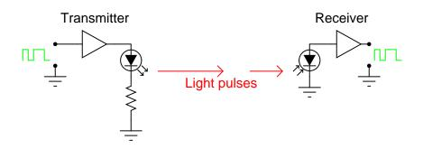
Transmitting digital information in optical form may be done in open air, simply by aiming a laser at a photodetector at a remote distance, but interference with the beam in the form of temperature inversion layers, dust, rain, fog, and other obstructions can present significant engineering problems:
