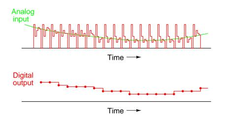
Note how the updates for this ADC occur at regular intervals, unlike the digital ramp ADC circuit.
