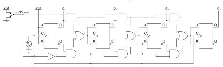
Up/down counter circuits are very useful devices. A common application is in machine motion control, where devices called *rotary shaft encoders* convert mechanical rotation into a series of electrical pulses, these pulses "clocking" a counter circuit to track total motion:
