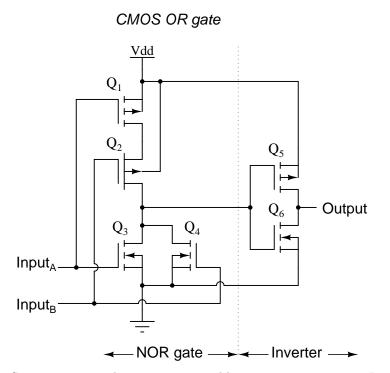
Since it appears that any gate possible to construct using TTL technology can be duplicated in CMOS, why do these two "families" of logic design still coexist? The answer is that both TTL and CMOS have their own unique advantages.
