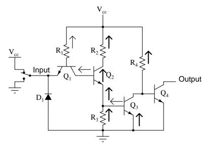
Having  $Q_2$  saturated causes  $Q_3$  to be saturated as well, resulting in very little voltage dropped between the base and emitter of the final output transistor  $Q_4$ . Thus,  $Q_4$  will be in cutoff mode, conducting no current. The output terminal will be floating (neither connected to ground nor  $V_{cc}$ ), and this will be equivalent to a "high" state on the input of the next TTL gate that this one feeds in to. Thus, a "high" input gives a "high" output.
