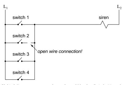
If this failure were to occur, the result would be that Switch #2 would no longer energize the siren if actuated. This, obviously, is not good in a fire alarm system. Unless the system were regularly tested (a good idea anyway), no one would know there was a problem until someone tried to use that switch in an emergency.
