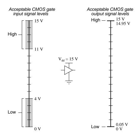
The margins for acceptable "high" and "low" signals may be greater than what is shown in the previous illustrations. What is shown represents "worst-case" input signal performance, based on manufacturer's specifications. In practice, it may be found that a gate circuit will tolerate "high" signals of considerably less voltage and "low" signals of considerably greater voltage than those specified here.
