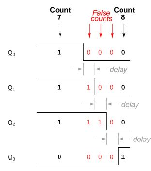
Instead of cleanly transitioning from a "0111" output to a "1000" output, the counter circuit will very quickly ripple from 0111 to 0110 to 0100 to 0000 to 1000, or from 7 to 6 to 4 to  $\theta$  and then to 8. This behavior earns the counter circuit the name of *ripple counter*, or *asynchronous counter*.
