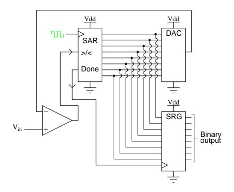
It should be noted that the SAR is generally capable of outputting the binary number in *serial* (one bit at a time) format, thus eliminating the need for a shift register. Plotted over time, the operation of a successive-approximation ADC looks like this:
