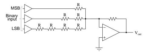
Unfortunately, this approach merely substitutes one type of complexity for another: volume of components over diversity of component values. There is, however, a more efficient design methodology.
