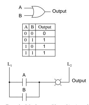
For each of the four possible combinations of input states (0-0, 0-1, 1-0, and 1-1), there is one, definite, unambiguous output state. Whether we're dealing with a multitude of cascaded gates or a single gate, that output state is determined by the truth table(s) for the gate(s) in the circuit, and nothing else.
