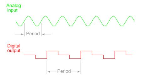
It should be understood that the Nyquist frequency is an *absolute* maximum frequency limit for an ADC, and does not represent the highest *practical* frequency measurable. To be safe, one shouldn't expect an ADC to successfully resolve any frequency greater than one-fifth to one-tenth of its sample frequency.
