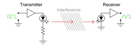
One way to avoid the problems of open-air optical data transmission is to send the light pulses down an ultra-pure glass fiber. Glass fibers will "conduct" a beam of light much as a copper wire will conduct electrons, with the advantage of completely avoiding all the associated problems of inductance, capacitance, and external interference plaguing electrical signals. Optical fibers keep the light beam contained within the fiber core by a phenomenon known as total internal reflectance.
