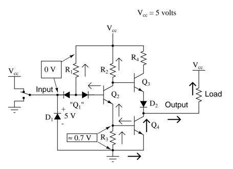
Inverter gate sinking current
