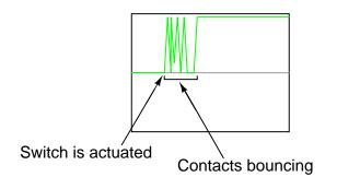
Close-up view of oscilloscope display:
