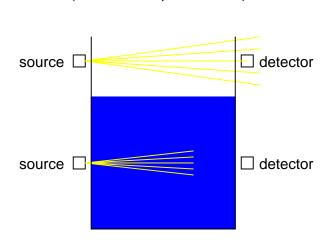
Nuclear level switch (for solid or liquid material)
