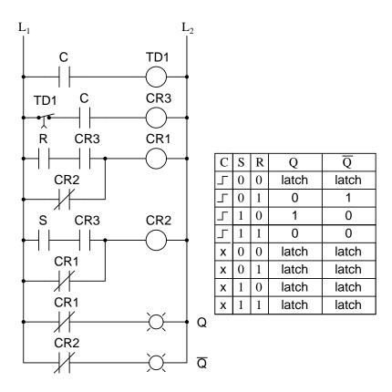
Relay contact  $CR_3$  in the ladder diagram takes the place of the old E contact in the S-R latch circuit, and is closed only during the short time that both C is closed and time-delay contact  $TR_1$  is closed. In either case (gate or ladder circuit), we see that the inputs S and R have no effect unless C is transitioning from a low (0) to a high (1) state. Otherwise, the flip-flop's outputs latch in their previous states.
