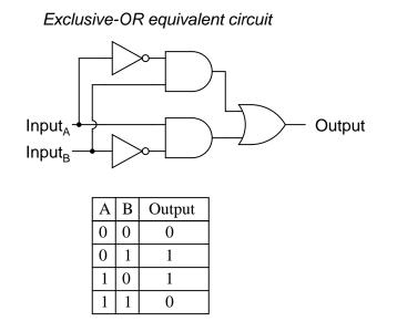
Exclusive-OR gates are very useful for circuits where two or more binary numbers are to be compared bit-for-bit, and also for error detection (parity check) and code conversion (binary to Grey and visa-versa).
