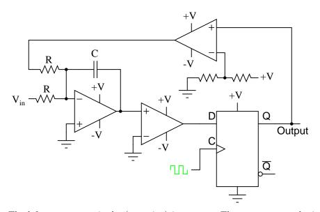
The leftmost op-amp is the (summing) integrator. The next op-amp the integrator feeds into is the comparator, or 1-bit ADC. Next comes the D-type flip-flop, which latches the comparator's output at every clock pulse, sending either a "high" or "low" signal to the next comparator at the top of the circuit. This final comparator is necessary to convert the single-polarity 0V / 5V logic level output voltage of the flip-flop into a +V / -V voltage signal to be fed back to the integrator.
