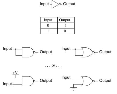
As you can see, there are two ways to use a NAND gate as an inverter, and two ways to use a NOR gate as an inverter. Either method works, although connecting TTL inputs together increases the amount of current loading to the driving gate. For CMOS gates, common input terminals decreases the switching speed of the gate due to increased input capacitance.
