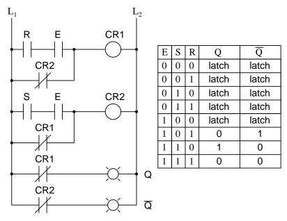
A practical application of this might be the same motor control circuit (with two normally-open pushbutton switches for *start* and *stop*), except with the addition of a master lockout input (E) that disables both pushbuttons from having control over the motor when it's low (0).
