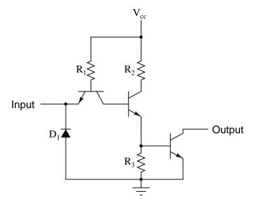
To designate open-collector output circuitry within a standard gate symbol, a special marker is used. Shown here is the symbol for an inverter gate with open-collector output:
