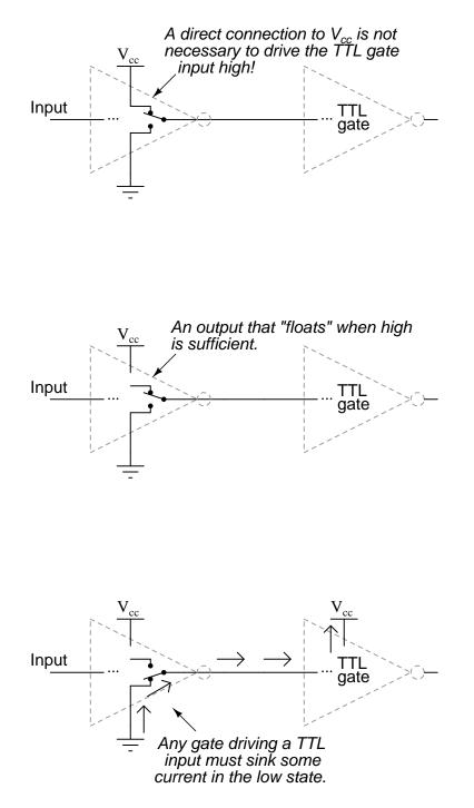
This means we have the option of simplifying the output stage of a gate circuit so as to eliminate  $Q_3$  altogether. The result is known as an *open-collector output*:
