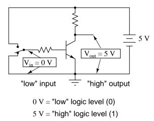
What we've created here with a single transistor is a circuit generally known as a *logic gate*, or
