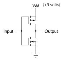
Notice the " $V_{dd}$ " label on the positive power supply terminal. This label follows the same convention as " $V_{cc}$ " in TTL circuits: it stands for the constant voltage applied to the drain of a field effect transistor, in reference to ground.
