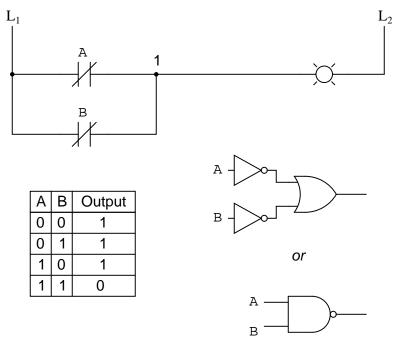
The lamp will be energized if *either* contact is unactuated. It will go out only if *both* contacts are actuated simultaneously.
