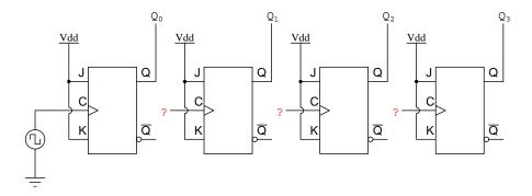
If we used flip-flops with negative-edge triggering (bubble symbols on the clock inputs), we could simply connect the clock input of each flip-flop to the Q output of the flip-flop before it, so that when the bit before it changes from a 1 to a 0, the "falling edge" of that signal would "clock" the next flip-flop to toggle the next bit: A four-bit "up" counter
