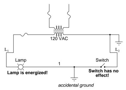
This time the accidental grounding of wire #1 will force power to the lamp while the switch will have no effect. It is much safer to have a system that blows a fuse in the event of a ground fault than to have a system that uncontrollably energizes lamps, relays, or solenoids in the event of the same fault. For this reason, the load(s) must always be located nearest the grounded power conductor in the ladder diagram.
