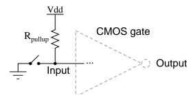
When switch is closed, the gate sees a definite "low" (0) input. When the switch is open,  $R_{pullup}$  will provide the connection to Vdd needed to secure a reliable "high" logic level for the CMOS gate input.
