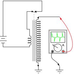
Borrowing terminology from the old mechanical buzzer (vibrator) circuits, solid-state circuit en-
