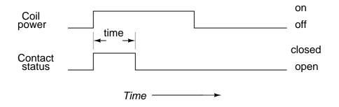
"Recycle" normally-open relay contact
