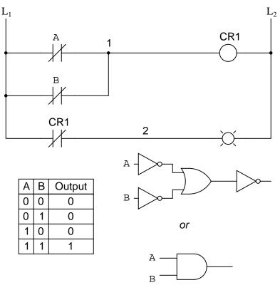
From the switches to the coil of  $CR_1$ , the logical function is that of a NAND gate.  $CR_1$ 's normallyclosed contact provides one final inversion to turn the NAND function into an AND function.
