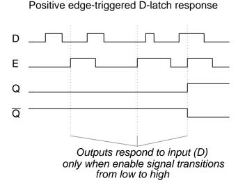
In the first timing diagram, the outputs respond to input D whenever the enable (E) input is high, for however long it remains high. When the enable signal falls back to a low state, the circuit remains latched. In the second timing diagram, we note a distinctly different response in the circuit output(s): it only responds to the D input during that brief moment of time when the enable signal *changes*, or *transitions*, from low to high. This is known as *positive* edge-triggering.
