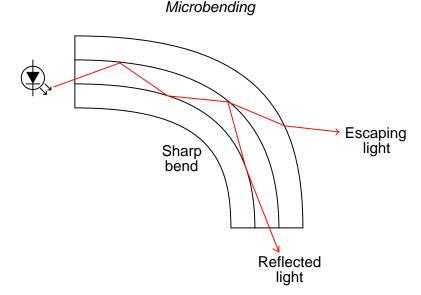
Not only does microbending lead to diminished signal strength due to the lost light, but it also constitutes a security weakness in that a light sensor intentionally placed on the outside of a sharp bend could intercept digital data transmitted over the fiber.
