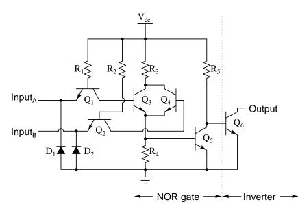
OR gate with open-collector output
