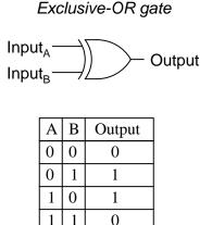
There are equivalent circuits for an Exclusive-OR gate made up of AND, OR, and NOT gates, just as there were for NAND, NOR, and the negative-input gates. A rather direct approach to simulating an Exclusive-OR gate is to start with a regular OR gate, then add additional gates to inhibit the output from going "high" (1) when both inputs are "high" (1):
