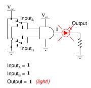
It is only with all inputs raised to "high" logic levels that the AND gate's output goes "high," thus energizing the LED for only one out of the four input combination states.
