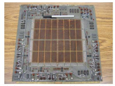
The electronic components seen around the periphery of this board are used for "driving" the column and row wires with current, and also to read the status of a core. A close-up photograph reveals the ring-shaped cores, through which the matrix wires thread. Again, a ball-point pen is shown for size comparison:
