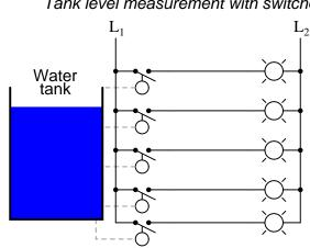
Tank level measurement with switches
