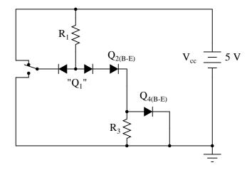
With the input switch in the "up" position (connected to  $V_{cc}$ ), it should be obvious that there will be no current through the left steering diode of  $Q_1$ , because there isn't any voltage in the switchdiode- $R_1$ -switch loop to motivate electrons to flow. However, there *will* be current through the right steering diode of  $Q_1$ , as well as through  $Q_2$ 's base-emitter diode junction and  $Q_4$ 's base-emitter diode junction:
