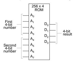
With 256 addressable memory locations in this ROM chip, we would have a fair amount of programming to do, telling it what binary output to generate for each and every combination of binary inputs. We would also run the risk of making a mistake in our programming and have it output an incorrect sum, if we weren't careful. However, the flexibility of being able to configure this function (or any function) through software alone generally outweighs that costs.
