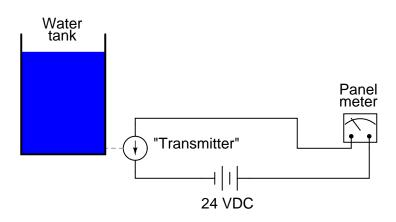
Analog tank-level measurement "loop"
