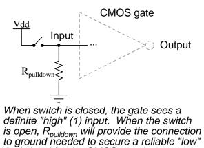
logic level for the CMOS gate input.
