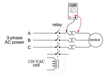
This is an especially useful trick to use for troubleshooting 3-phase AC motors, to see if one phase winding is burnt open or disconnected, which will result in a rapidly destructive condition known as "single-phasing." If one of the lines carrying power to the motor is open, it will not have any current through it (as indicated by a 0.00 mV reading across its heater), although the other two lines will (as indicated by small amounts of voltage dropped across the respective heaters).
