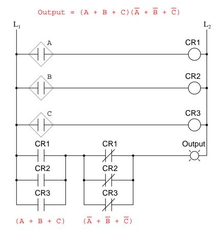
The previous two circuits represent different versions of the "sensor disagreement" logic circuit only, not the "good flame" detection circuit(s). The entire logic system would be the combination of both "good flame" and "sensor disagreement" circuits, shown on the same diagram.
