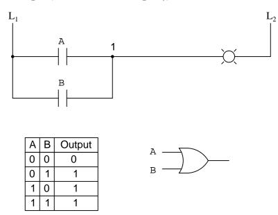
Now, the lamp will come on if either contact A or contact B is actuated, because all it takes for the lamp to be energized is to have at least one path for current from wire  $L_1$  to wire 1. What we have is a simple OR logic function, implemented with nothing more than contacts and a lamp.
