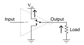
Please note that this two-position switch shown inside the gate symbol is representative of transistors  $Q_3$  and  $Q_4$  alternately connecting the output terminal to  $V_{cc}$  or ground, *not* of the switch previously shown sending an input signal to the gate!
