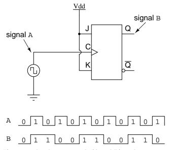
If we consider the two signals (A and B) in this circuit to represent two bits of a binary number, signal A being the LSB and signal B being the MSB, we see that the count sequence is backward: from 11 to 10 to 01 to 00 and back again to 11. Although it might not be counting in the direction we might have assumed, at least it counts!
