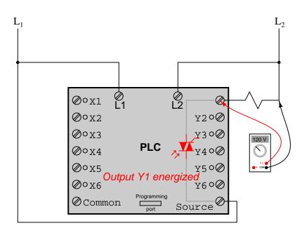
In this way, the PLC is able to interface with real-world devices such as switches and solenoids.
