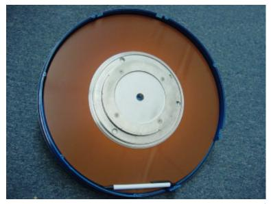
Modern disk drives use multiple platters made of hard material (hence the name, "hard drive") with multiple read/write heads for every platter. The gap between head and platter is much smaller than the diameter of a human hair. If the hermetically-sealed environment inside a hard disk drive is contaminated with outside air, the hard drive will be rendered useless. Dust will lodge between the heads and the platters, causing damage to the surface of the media.
