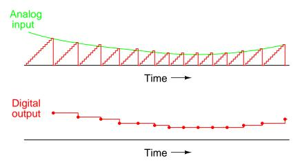
Note how the time between updates (new digital output values) changes depending on how high the input voltage is. For low signal levels, the updates are rather close-spaced. For higher signal levels, they are spaced further apart in time:
