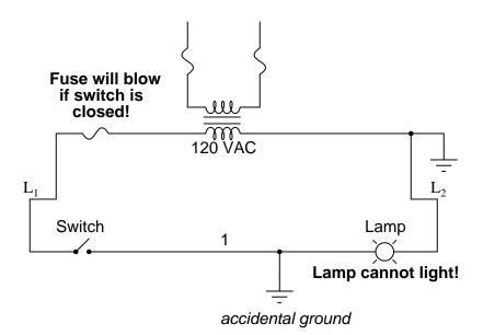
With both sides of the lamp connected to ground, the lamp will be "shorted out" and unable to receive power to light up. If the switch were to close, there would be a short-circuit, immediately blowing the fuse.
