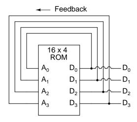
The above circuit illustrates the basic idea: the data stored at each address becomes the next storage location that the ROM gets addressed to. The result is a specific sequence of binary numbers (following the sequence programmed into the ROM) at the output, over time. To avoid signal timing problems, though, we need to connect the data outputs back to the address inputs through a 4-bit D-type flip-flop, so that the sequence takes place step by step to the beat of a controlled clock pulse:
