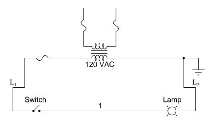
Here, the lamp (load) is located on the right-hand side of the rung, and so is the ground connection for the power source. This is no accident or coincidence; rather, it is a purposeful element of good design practice. Suppose that wire #1 were to accidently come in contact with ground, the insulation of that wire having been rubbed off so that the bare conductor came in contact with grounded, metal conduit. Our circuit would now function like this:
