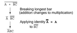
As a result, the original circuit is reduced to a three-input AND gate with the A input inverted:
