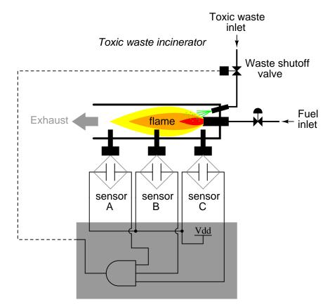
If using relay circuitry, we could create this AND function by wiring three relay contacts in series, or simply by wiring the three sensor contacts in series, so that the only way electrical power could be sent to open the waste valve is if all three sensors indicate flame:
