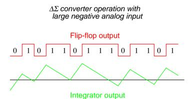
A parallel binary number output is obtained from this circuit by averaging the serial stream of bits together. For example, a counter circuit could be designed to collect the total number of 1's output by the flip-flop in a given number of clock pulses. This count would then be indicative of the analog input voltage.
