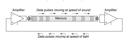
Mercury tube delay-line memory
