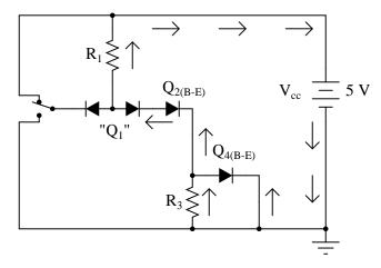
This tells us that in the real gate circuit, transistors  $Q_2$  and  $Q_4$  will have base current, which will turn them on to conduct collector current. The total voltage dropped between the base of  $Q_1$ (the node joining the two back-to-back steering diodes) and ground will be about 2.1 volts, equal to the combined voltage drops of three PN junctions: the right steering diode,  $Q_2$ 's base-emitter diode, and  $Q_4$ 's base-emitter diode.
