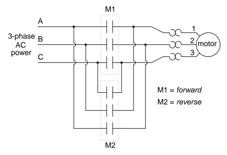
When contactor  $M_1$  is energized, the 3 phases (A, B, and C) are connected directly to terminals 1, 2, and 3 of the motor, respectively. However, when contactor  $M_2$  is energized, phases A and B are reversed, A going to motor terminal 2 and B going to motor terminal 1. This reversal of phase wires results in the motor spinning the opposite direction. Let's examine the control circuit for these two contactors:
