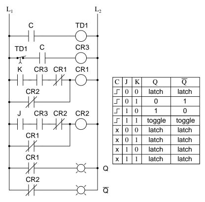
The end result is that the S-R flip-flop's "invalid" state is eliminated (along with the race condition it engendered) and we get a useful feature as a bonus: the ability to toggle between the two (bistable) output states with every transition of the clock input signal.
