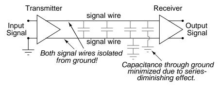
The triangular amplifier symbols represent *differential amplifiers*, which output a voltage signal between two wires, neither one electrically common with ground. Having eliminated any relation between the voltage signal and ground, the only significant capacitance imposed on the signal voltage is that existing between the two signal wires. Capacitance between a signal wire and a grounded conductor is of much less effect, because the capacitive path between the two signal wires via a
