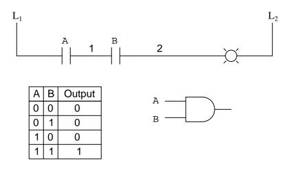
Now, the lamp energizes only if contact A and contact B are simultaneously actuated. A path exists for current from wire  $L_1$  to the lamp (wire 2) if and only if *both* switch contacts are closed.
