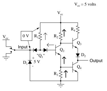
With base current provided, transistor  $Q_2$  will be turned "on." More specifically, it will be *saturated* by virtue of the more-than-adequate current allowed by  $R_1$  through the base. With  $Q_2$  saturated, resistor  $R_3$  will be dropping enough voltage to forward-bias the base-emitter junction of transistor  $Q_4$ , thus saturating it as well:
