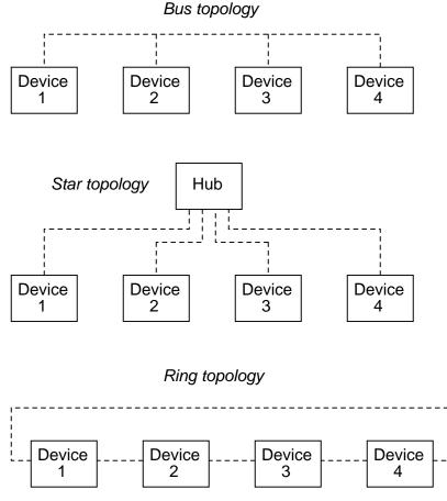
Many network standards dictate the type of topology which is used, while others are more versatile. Ethernet, for example, is commonly implemented in a "bus" topology but can also be implemented in a "star" or "ring" topology with the appropriate interconnecting equipment. Other networks, such as RS-232C, are almost exclusively point-to-point; and token ring (as you might have guessed) is implemented solely in a ring topology.
