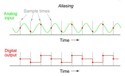
Note how the period of the output waveform is much longer (slower) than that of the input waveform, and how the two waveform shapes aren't even similar:
