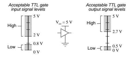
If a voltage signal ranging between 0.8 volts and 2 volts were to be sent into the input of a TTL gate, there would be no certain response from the gate. Such a signal would be considered *uncertain*, and no logic gate manufacturer would guarantee how their gate circuit would interpret such a signal.
