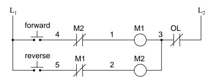
Now, when  $M_1$  is energized, the normally-closed auxiliary contact on the second rung will be open, thus preventing  $M_2$  from being energized, even if the "Reverse" pushbutton is actuated. Likewise,  $M_1$ 's energization is prevented when  $M_2$  is energized. Note, as well, how additional wire numbers (4 and 5) were added to reflect the wiring changes.
