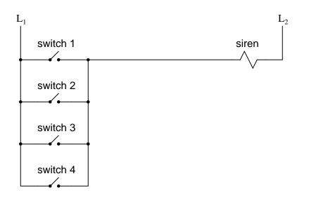
Essentially, this is the OR logic function implemented with four switch inputs. We could expand this circuit to include any number of switch inputs, each new switch being added to the parallel network, but I'll limit it to four in this example to keep things simple. At any rate, it is an elementary system and there seems to be little possibility of trouble.
