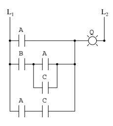
As before, our first step in reducing this circuit to its simplest form must be to develop a Boolean expression from the schematic. The easiest way I've found to do this is to follow the same steps I'd normally follow to reduce a series-parallel resistor network to a single, total resistance. For example, examine the following resistor network with its resistors arranged in the same connection pattern as the relay contacts in the former circuit, and corresponding total resistance formula:
