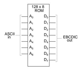
Again, all that is required is for the ROM chip to be properly programmed with the necessary data so that each valid ASCII input will produce a corresponding EBCDIC output code.
