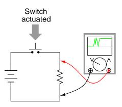
A closer look at the oscilloscope display reveals a rather ugly set of makes and breaks when the switch is actuated a single time:
