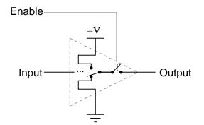
With the enable input held "high" (1), the buffer acts like an ordinary buffer with a totem pole output stage: it is capable of both sourcing and sinking current. However, the output terminal floats (goes into "high-Z" mode) if ever the enable input is grounded ("low"), regardless of the data signal's logic level. In other words, making the enable input terminal "low" (0) effectively *disconnects* the gate from whatever its output is wired to so that it can no longer have any effect.
