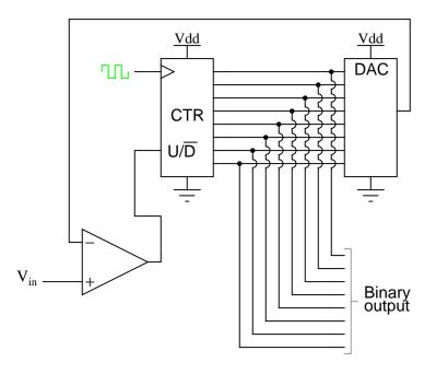
Notice how no shift register is needed to buffer the binary count at the end of a cycle. Since the counter's output continuously tracks the input (rather than counting to meet the input and then resetting back to zero), the binary output is legitimately updated with every clock pulse.
