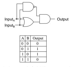
In this circuit, the final AND gate acts as a buffer for the output of the OR gate whenever the NAND gate's output is high, which it is for the first three input state combinations (00, 01, and 10). However, when both inputs are "high" (1), the NAND gate outputs a "low" (0) logic level, which forces the final AND gate to produce a "low" (0) output.
