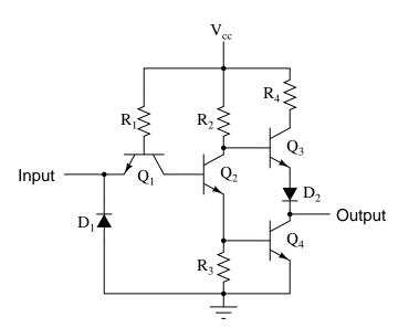
This circuit is composed exclusively of resistors and bipolar transistors. Bear in mind that other circuit designs are capable of performing the NOT gate function, including designs substituting field-effect transistors for bipolar (discussed later in this chapter).
