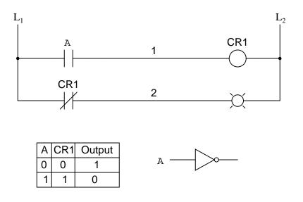
We will call the relay, "control relay 1," or  $CR_1$ . When the coil of  $CR_1$  (symbolized with the pair of parentheses on the first rung) is energized, the contact on the second rung *opens*, thus deenergizing the lamp. From switch A to the coil of  $CR_1$ , the logic function is noninverted. The normally-closed contact actuated by relay coil  $CR_1$  provides a logical inverter function to drive the lamp opposite that of the switch's actuation status.
