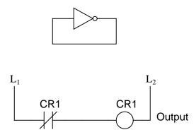
When the input is 0, the output switches to 1. That 1 output gets fed back to the input as a 1. When the input is 1, the output switches to 0. That 0 output gets fed back to the input as a 0, and the cycle repeats itself. The result is a high frequency (several megahertz) oscillator, if implemented with a solid-state (semiconductor) inverter gate:
