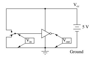
Power supply conductors are rarely shown in gate circuit schematics, even if the power supply connections at each gate are. Minimizing lines in our schematic, we get this:
