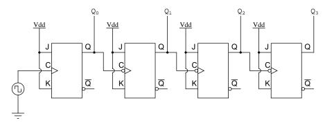
This circuit would yield the following output waveforms, when "clocked" by a repetitive source of pulses from an oscillator:
