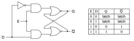
Note that the R input has been replaced with the complement (inversion) of the old S input, and the S input has been renamed to D. As with the gated S-R latch, the D latch will not respond to a signal input if the enable input is 0 - it simply stays latched in its last state. When the enable input is 1, however, the Q output follows the D input.
