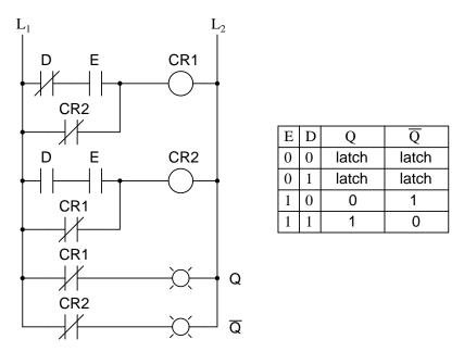
An application for the D latch is a 1-bit memory circuit. You can "write" (store) a 0 or 1 bit in this latch circuit by making the enable input high (1) and setting D to whatever you want the stored bit to be. When the enable input is made low (0), the latch ignores the status of the D input and merrily holds the stored bit value, outputting at the stored value at Q, and its inverse on output not-Q.
