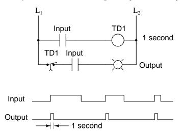
No matter how long the input signal stays high (1), the output remains high for just 1 second of time, then returns to its normal (stable) low state.
