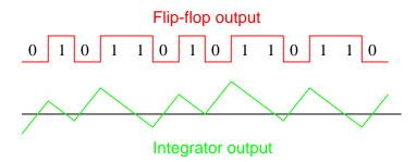
As the analog input signal increases in magnitude, so does the occurrence of 1's in the digital output of the flip-flop:
