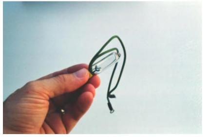
Mercury switch contacts are impractical to build in large sizes, and so you will typically find such contacts rated at no more than a few amps, and no more than 120 volts. There are exceptions, of course, but these are common limits.
