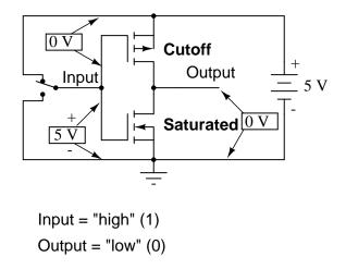
Now the lower transistor (N-channel) is saturated because it has sufficient voltage of the correct polarity applied between gate and substrate (channel) to turn it on (positive on gate, negative on the channel). The upper transistor, having zero voltage applied between its gate and substrate, is in its normal mode: *off*. Thus, the output of this gate circuit is now "low" (0). Clearly, this circuit exhibits the behavior of an inverter, or NOT gate.
