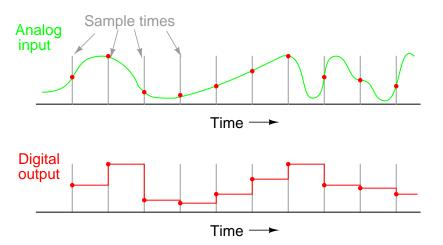
When the sample period is too long (too slow), substantial details of the analog signal will be missed. Notice how, especially in the latter portions of the analog signal, the digital output utterly fails to reproduce the true shape. Even in the first section of the analog waveform, the digital
