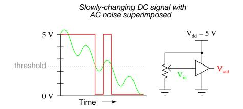
If this scenario looks familiar to you, it's because you remember a similar problem with (analog) voltage comparator op-amp circuits. With a single threshold point at which an input causes the output to switch between "high" and "low" states, the presence of significant noise will cause erratic changes in the output:
