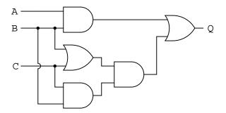
Our first step in simplification must be to write a Boolean expression for this circuit. This task is easily performed step by step if we start by writing sub-expressions at the output of each gate, corresponding to the respective input signals for each gate. Remember that OR gates are equivalent to Boolean addition, while AND gates are equivalent to Boolean multiplication. For example, I'll write sub-expressions at the outputs of the first three gates:
