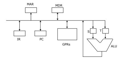
The ALU, the bus and all the registers in the data path are of identical size. All operations including incrementation of the PC and the GPRs are to be carried out in the ALU. Two clock cycles are needed for memory read operation – the first one for loading
