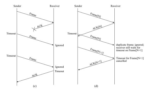
Here is the version of Fig 3.15(c) (lost ACK), showing a receiver timeout of approximately half the sender timeout.
