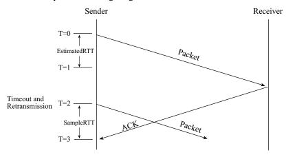
To get to such a steady state, assume that originally RTT = EstimatedRTT = 1.45, say, and RTT then jumps to 3.0 as above. The first packet sent under the new rules will time out and be retransmitted at T=2.9; when the ACK arrives at T=3.0 we record SampleRTT = 0.1. This causes EstimatedRTT to decrease. It will continue to grow smaller, monotonically (at least if  $\beta$  is not too large), converging on the value 1.0 as above.
