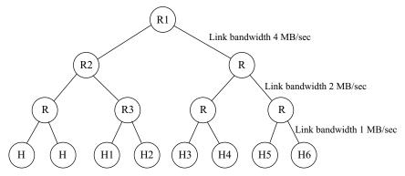
We arrange for H3 and H4 to send 1MB/sec to H1, and H5 and H6 to send 1MB/sec to H2. Each of the links to the right of R1 reaches its maximum capacity, as does the R1—R2 link,
