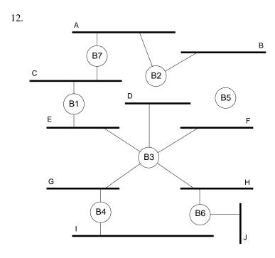
13. When A sends to C, all bridges see the packet and learn where A is. However, when C then sends to A, the packet is routed directly to A and B4 does not learn where C is. Similarly, when D sends to C, the packet is routed by B2 towards B1 only, and B1 does not learn where D is.
