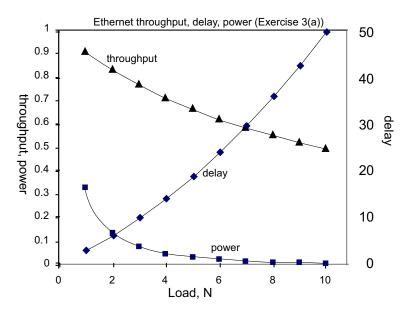
Both power curves have their maximum at N=1, the minimum N, which is somewhat artificial and is an artifact of the unnatural way we are measuring load.
