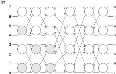
33. We simply connect the output wires from the bottom-left  $4 \times 4$  sub-Batcher sorter (the bottom-left  $2 \times 3$  block of switching elements) in the reverse order of the way they were originally connected to the merger section. The unreversed sub-Batcher sorts its output in increasing order; by reversing the wires this output enters column 4 in decreasing order as desired.
