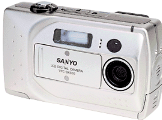
FIGURE 7.44 The Sanyo VPC-SX500. Although newer cameras offer more pixels per picture, the principles are the same. This 1360 x 1024 pixel digital camera stores pictures either using Compact Flash memory, which ranges from 8 MB to 64 MB, or using a 340 MB IBM Microdrive. It is 4.3" wide x 2.5" high x 1.6" deep, and it weighs 7.4 ounces. In addition to taking still picture and converting it to JPEG format every 0.9 seconds, it can record a Quick Time video clip at VGA Size (640 x 480). Using the IBM Microdrive, it can record up to 7.5 minutes at 15 frames per second with sound (10,000 images) or 50 minutes for 160 x 120 pixel video with sound. Without video, it can record up to 12 hours of 8-bit 8 KHz audio. The Flash memory storage capacity is 5X to 40X shorter, so its video and audio capacity are also 5X to 40X smaller. One technological advantage is the use of a custom system on a chip to reduce size and power, so the camera only needs two AA batteries to operate versus four in other digital cameras.
