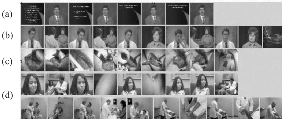
Figure 4. Semantic Scene Generation Results for Medical Videos where the Discriminable Regions such as Slide, Clipart, Blood-Red, Skin-Color, Human Faces, etc., are First Detected [These discriminable regions are then grouped into four semantic scenes according to pre-defined models (domain knowledge): (a) presentation, (b) dialog, (c) surgery, and (d) diagnosis.]
