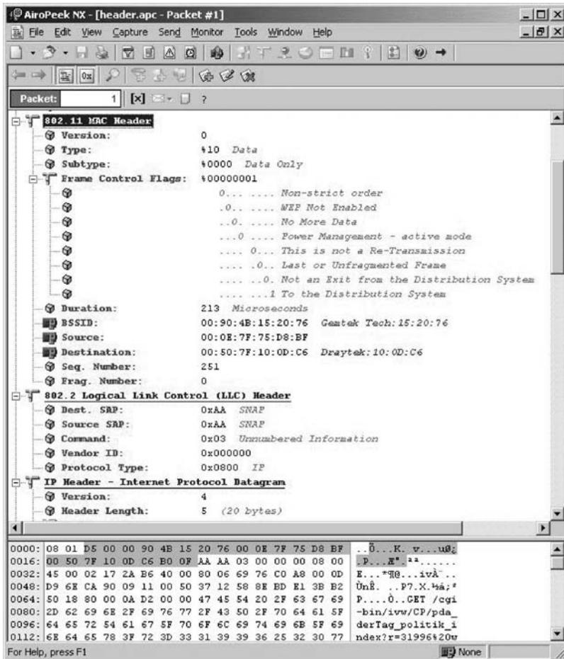
Figure 4.13 MAC and LLC header of a WLAN frame
