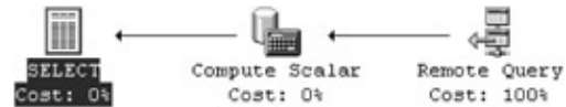
Figure 13–11: Execution plan for a SELECT * WHERE CustomerID = 'WILMK' OR CustomerID = 'WOLZA' statement against a federated view
