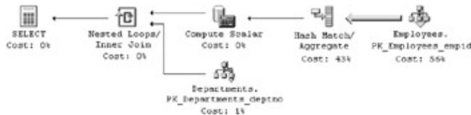
Figure 8–6: Execution plan for an aggregate query with no covering index or indexed view A full clustered index scan is performed on the PK_Employees_empid index, followed by a hash match aggregate that calculates the aggregations for each deptno, followed by a nested loop join with the Departments table to retrieve the deptname column. Currently there is a clustered index on the empid column in the Employees table, as well as a clustered index on the deptno column in the Departments table. You don't have an index on the Employees table that will allow the optimizer to avoid a full clustered index scan on it. The I/O cost of this query is quite large because all of the clustered index pages (the data pages in the large Employees table) are scanned, as shown in Listing 8–41.
