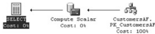
Figure 13–8: Execution plan for a SELECT * WHERE CustomerID = 'ALFKI' statement against a federated view
