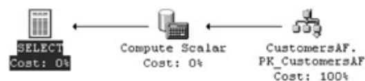
Figure 13–10: Execution plan for a SELECT * WHERE CustomerID = 'ALFKI' OR CustomerID = 'ANATR' statement against a federated view
